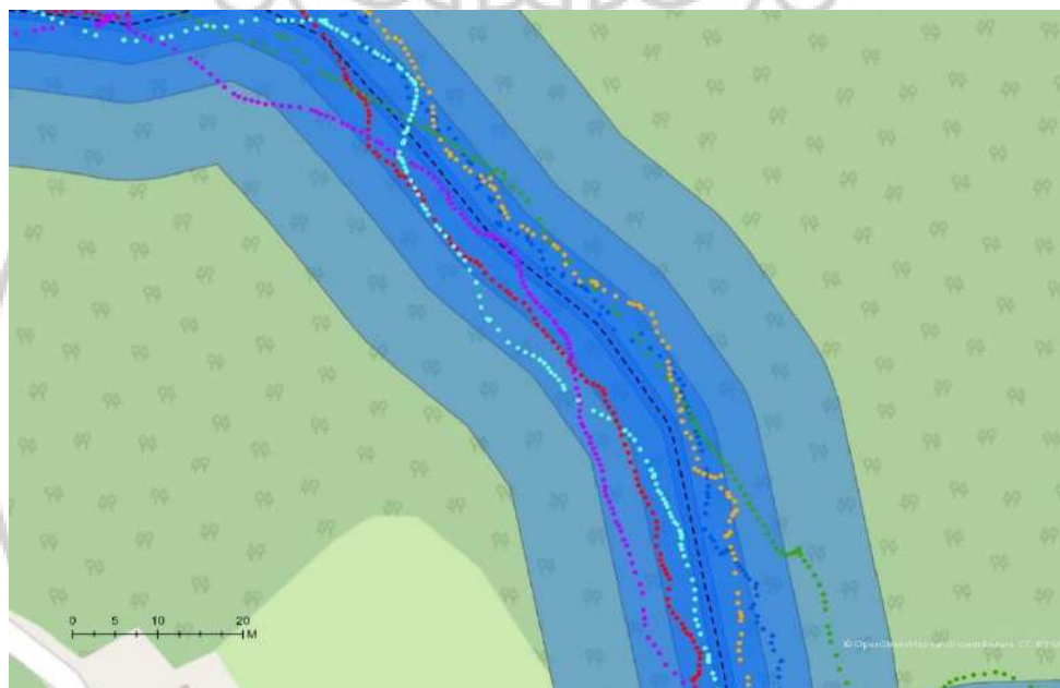
Figure 2. Conceptual illustration of the buffer-based method used for horizontal positional accuracy assessment. A reference trail geometry derived from OpenStreetMap (OSM) is surrounded by concentric buffer zones of increasing width (1 m, 5 m, 10 m and 20 m). GPS track points fall inside or outside each buffer.
